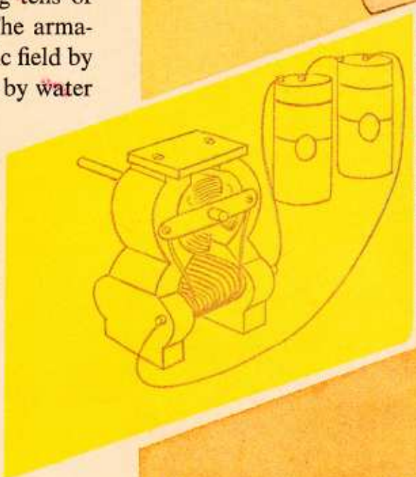
Above, closeup of a toy motor connected to two dry cells (batteries).
